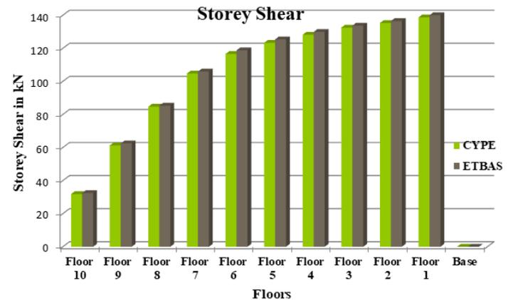
Fig 4.5: Storey shear for 10mm thick SPSW
