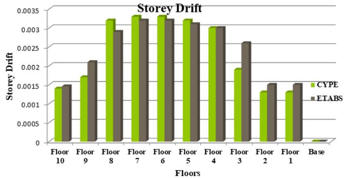
Fig 4.3: Storey drift for 10mm thick SPSW
