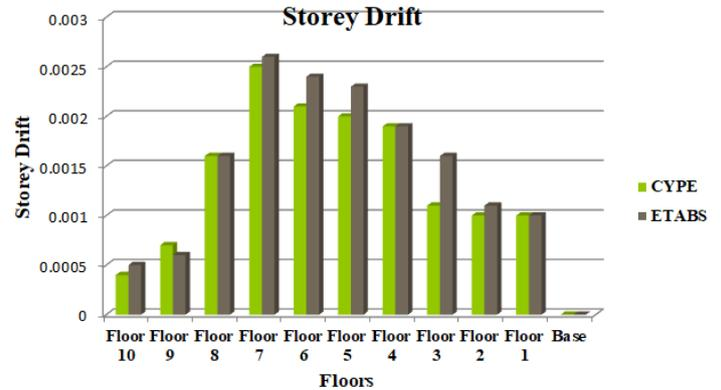
Fig 4.4: Storey drift for 50mm thick SPSW
