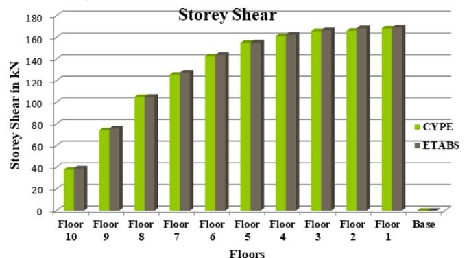
Fig 4.6: Storey shear for 50mm thick SPSW
