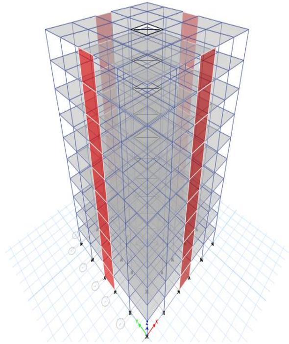
Fig 2.5:Elevation view of the structure in ETAB software
