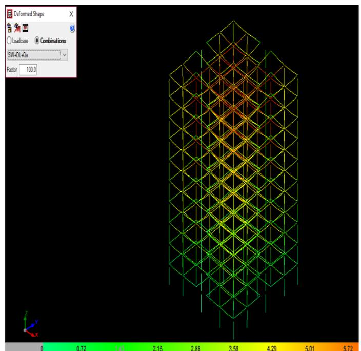
Fig 3.1:Deflection Diagram of structure in CYPE software
