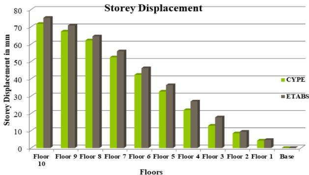
Fig 4.1: Maximum displacement for 10mm thick SPSW
