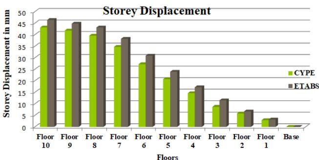
Fig 4.2: Maximum displacement for 50mm thick SPSW
