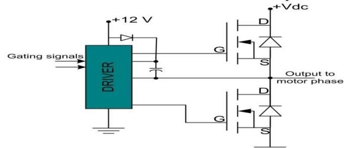
The FAN7392 is a monolithic high- and low-side gate drive IC, that can drive high-speed MOSFETs and IGBTs that operate up to +600V. It has a buffered output stage with all NMOS transistors designed for high pulse current driving capability and minimum cross-conduction. Fairchild’s high-voltage process and common-mode noise canceling techniques provide stable operation of the high-side driver under high dv/dt noise circumstances. An advanced level-shift circuit
