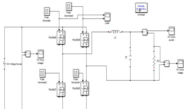
Simulation model of single phase inverter using MATLAB Simulink Software.
