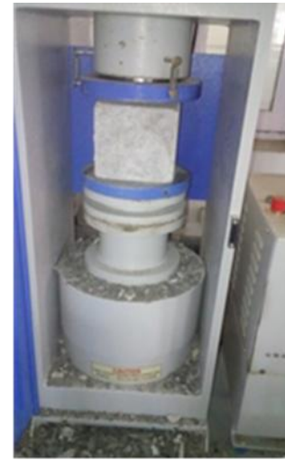
FIGUREV COMPRESSION TESTING ON CUBES
