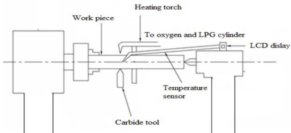
Between machine headstock and tail stock, and before device carriage the apparatus is mounted. Fig.9 Experimental Setup This trial setup for the most part comprises of eight vital segments and they are as per the following:-
