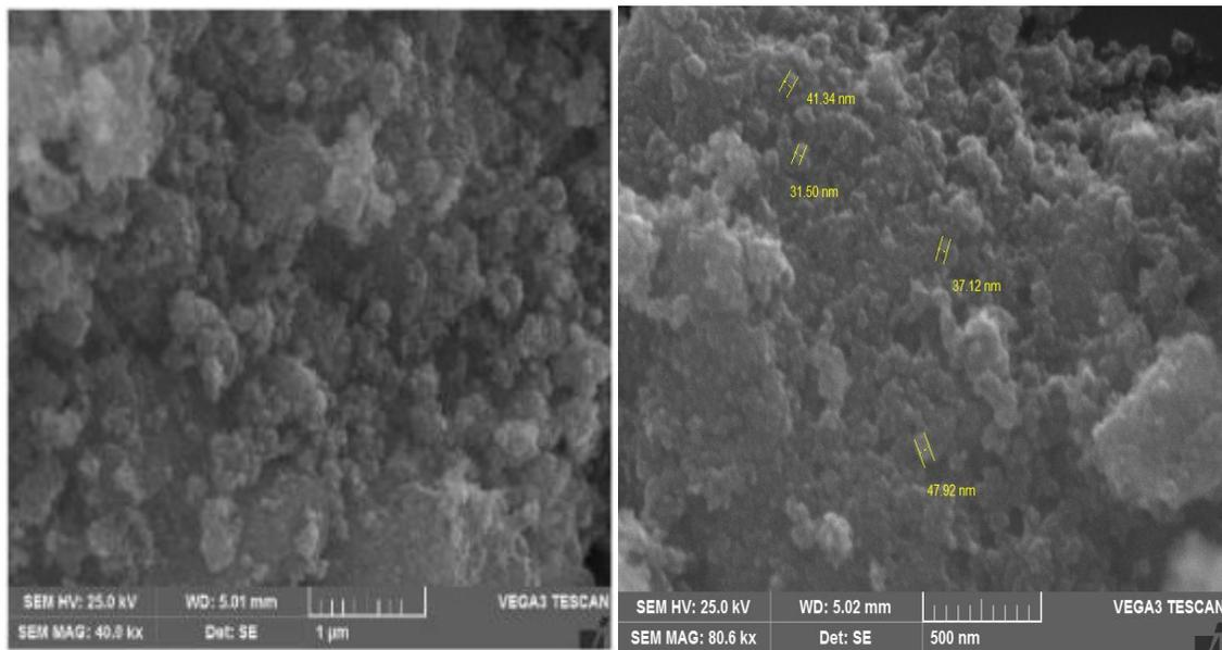
**Figure.2. The SEM image of TiO<sub>2</sub> doped Fe<sub>3</sub>O<sub>4</sub>nanoparticles.**
