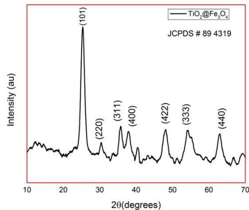
**Figure.1. the X-ray Diffraction pattern of TiO<sub>2</sub> doped Fe<sub>3</sub>O<sub>4</sub>nanoparticles**
