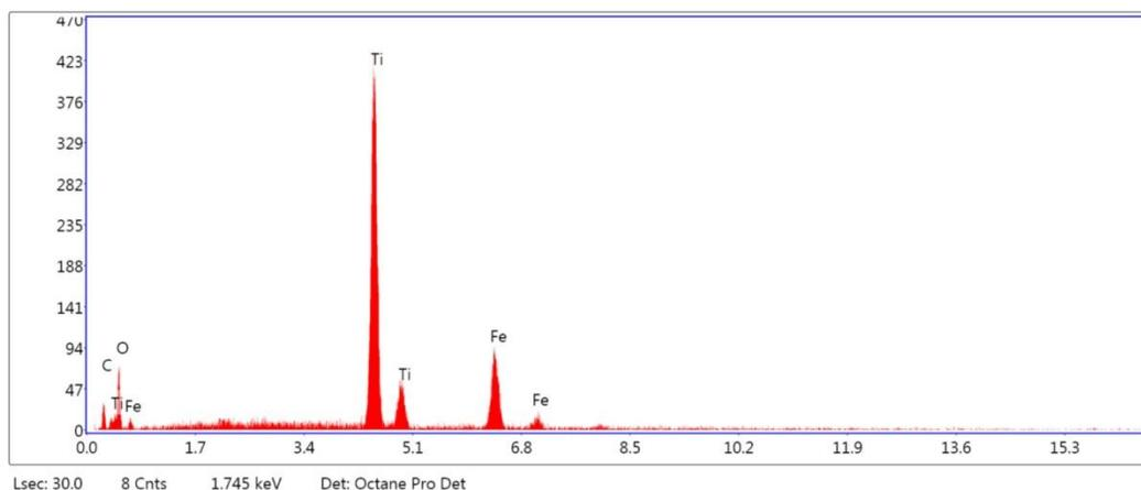
**Figure.3. EDAX image of TiO<sub>2</sub> doped Fe<sub>3</sub>O<sub>4</sub>nanoparticles**
