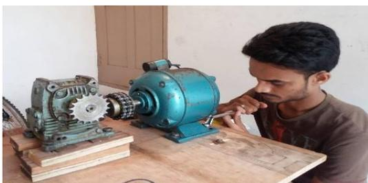
Figure.5. assembly of worm gearbox with motor on mounting frame.
