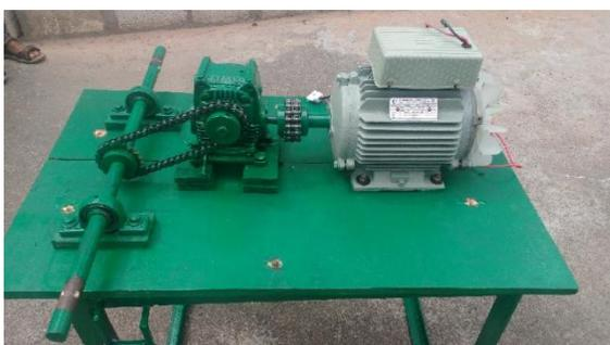
Figure.6. assembly of worm gearbox, chain drive with main shaft on mounting frame.
