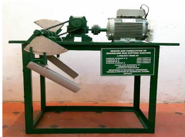
Figure.8. final assembly of sugarcane bud cutting machine
