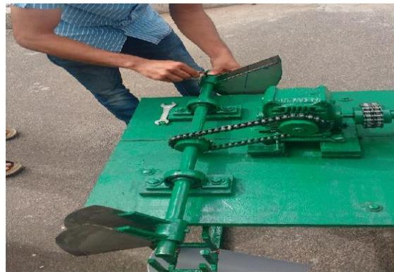
Figure.7. assembly of cutting blade with main shaft on mounting frame
