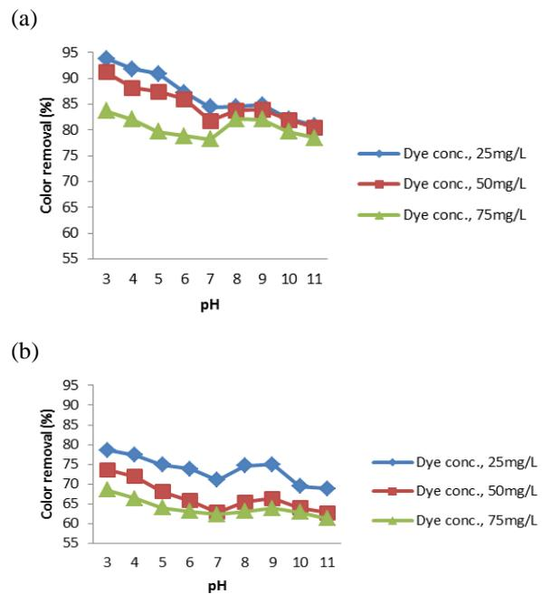
**Figure.2. Effect of pH on color removal at different dye concentration (WTR dose 100mg/L) (a) for cationic dye (b) for anionic dye**
