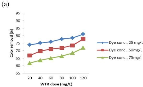
(a) (b) **Figure. 1 Effect of WTR dose on color removal on different dye concentration (initial pH 3.0) (a) for cationic dye (b) for anionic dye**
