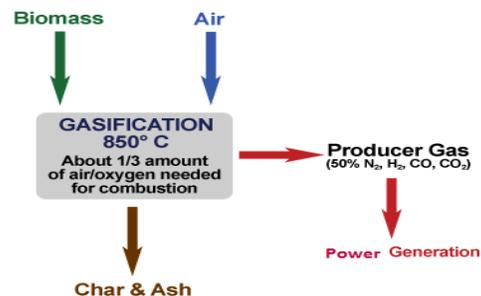
Figure.3. Biomass Gasification via Partial Oxidation (Auto Thermal)
