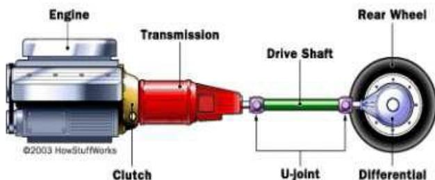
Figure.1. Location of Propeller/Drive Shaft
