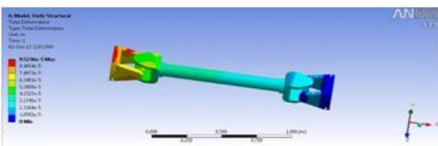
Figure.8. Total deformation (carbon fibre).
