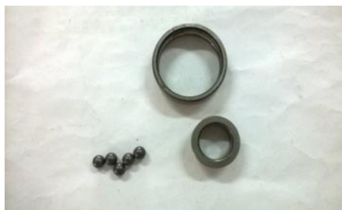
Figure.3. Damage ball bearing.
