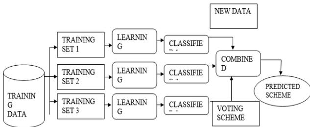
**Figure.2. Flowchart of Bagging Classifier**
