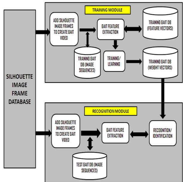
FIG. 1. GENERALIZED FRAMEWORK OF GAIT RECOGNITION.
