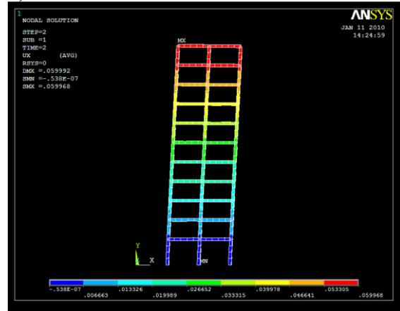
**b) Deformed profile of the frame**
