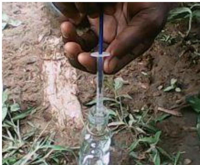
Plate 5: Injection of  $MnSO_4$  (Reagent) into Water Sample to Retain Oxygen Prior Analysis.
