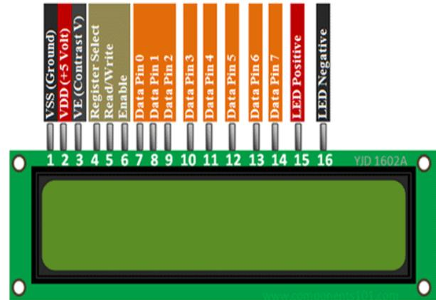
Figure.4. 16x2 LCD display.
