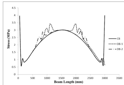
Figure.19. Stress distribution along length for CB, DB-1, DB-2
