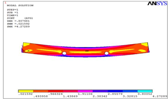
Figure .16. Contour plot of stress intensity of DB1
