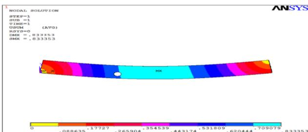
**Figure .5. Contour Plot of Displacement of SB1**
