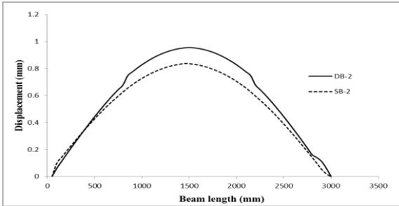
Figure .12. Comparison of Displacement between SB-2 and DB-2
