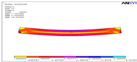
Figure .13. Contour plot of stress intensity of CB
