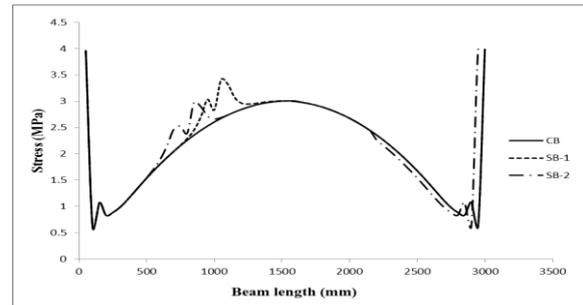
Figure .18. Stress distribution along length for CB, SB-1, SB-2
