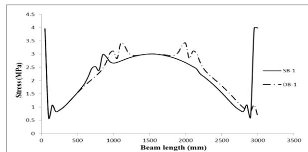
Figure. 20. Stress distribution along length for SB-1, DB-1
