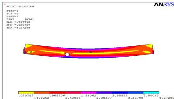
Figure .14. Contour plot of stress intensity of SB1
