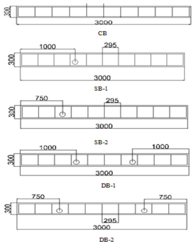
**Figure.3. Beam cases (All dimensions are in mm)**
