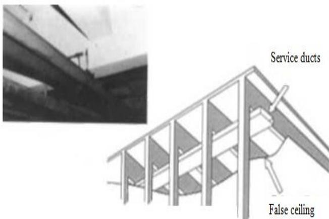
**Figure.1. Typical layouts of service ducts and pipes**
