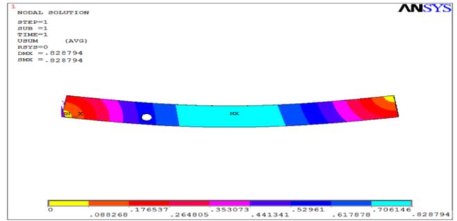
**Figure 6. Contour Plot of Displacement of SB2**
