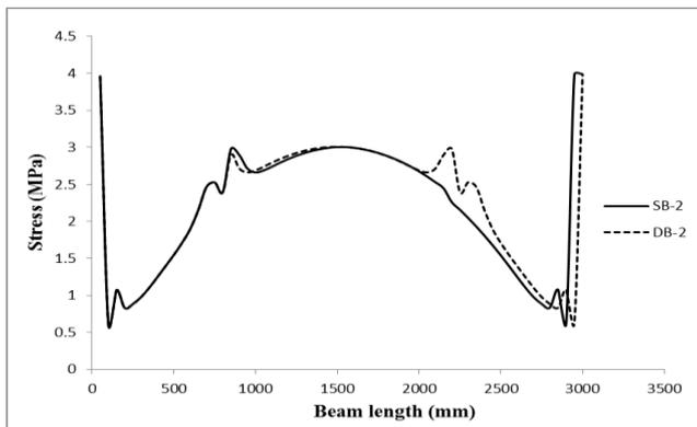
**Figure .21. Stress distribution along length for SB-2, DB-2**
