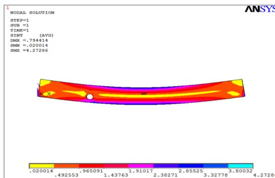
Figure. 15. Contour plot of stress intensity of SB2
