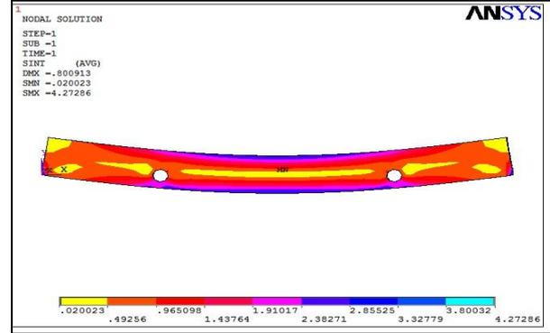
Figure .17. Contour plot of stress intensity of DB2
