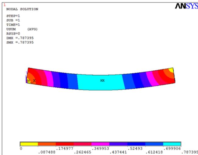
**Figure .4. Contour Plot of Displacement of CB**
