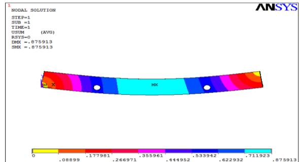
**Figure 8. Contour Plot of Displacement of DB2**
