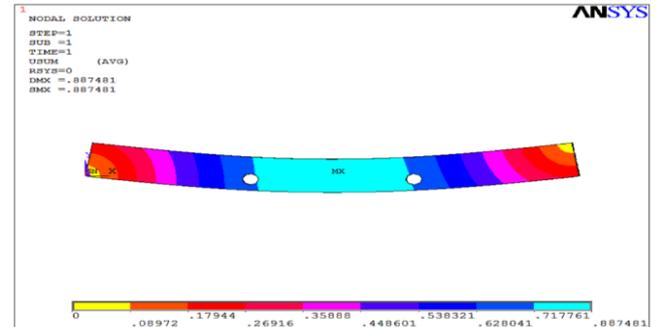
**Figure .7. Contour Plot of Displacement of DB1**
