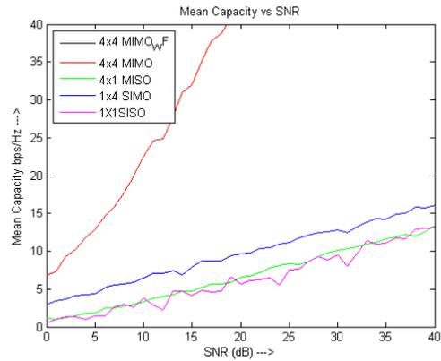
**Figure.4. Comparison of Multi-user achievable rates with SISO SIMO MISO in Rayleigh fading environments.**
