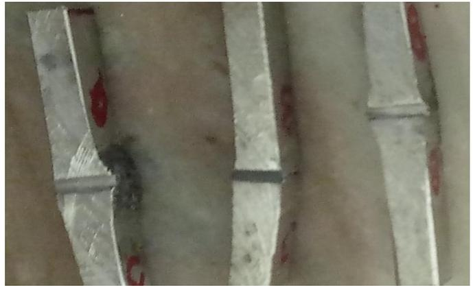
Figure .4. Impact Test Samples
