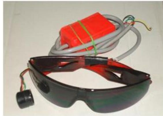
Figure.3. IR Based Eye Blink Sensor
