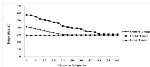
**Figure.15. Discharging PCM Temperature with respect to Time for flow rate of 20 lit/hr of Palmitic acid**
