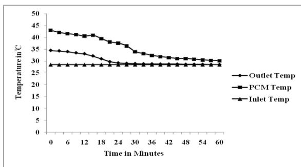
**Figure.12. Discharging PCM Temperature with respect to Time for flow rate of 15 lit/hr of Myristic acid**
