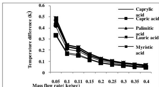
Figure.3. Variation of Temperature Difference with respect to Mass Flow Rate for Various PCM.
