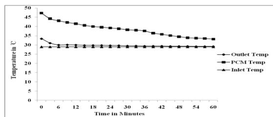
Figure.7. Discharging PCM Temperature with respect to Time for flow rate of 20 lit/hr of Lauric acid
