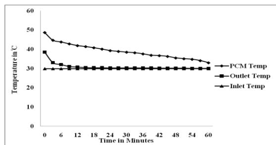
Figure.8. Discharging PCM Temperature with respect to Time for flow rate of 15 lit/hr of Lauric acid
