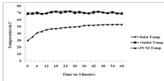
**Figure.14. Charging PCM Temperature with respect to Time for flow rate of 15 lit/hr of Palmitic acid**
