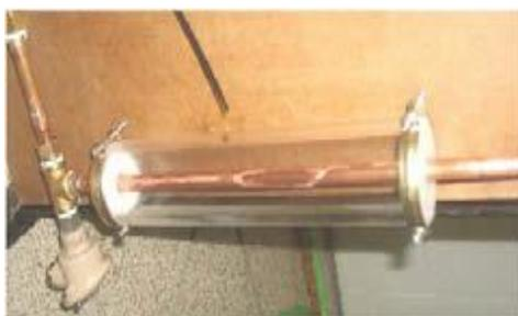
**Figure.1. Double pipe copper tube heat exchanger**
