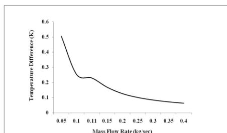
Figure.2. Variation of Temperature Difference with respect to Mass Flow Rate for Myristic Acid.
