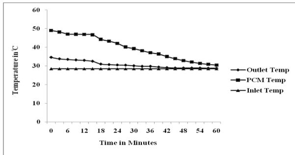
**Figure.11. Discharging PCM Temperature with respect to Time for flow rate of 20 lit/hr of Myristic acid**
