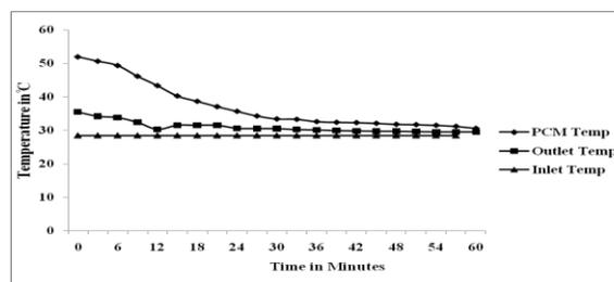
**Figure.16. Discharging PCM Temperature with respect to Time for flow rate of 15 lit/hr of Palmitic acid**
