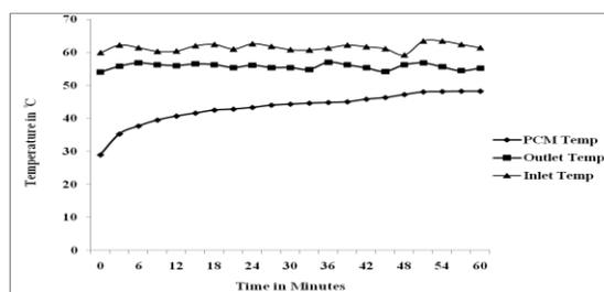
Figure.6. Charging PCM Temperature with respect to Time for flow rate of 15 lit/hr of Lauric acid
