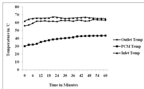
Figure.10. Charging PCM Temperature with respect to Time for flow rate of 15 lit/hr of Myristic acid
