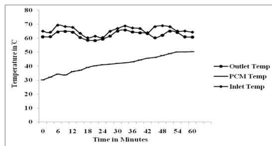
Figure.9. Charging PCM Temperature with respect to Time for flow rate of 20 lit/hr of Myristic acid
