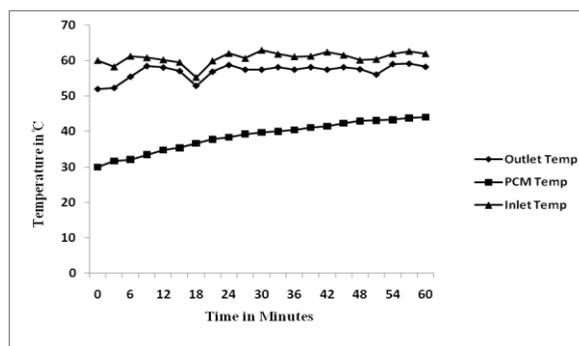
Figure.5. Charging PCM Temperature with respect to Time for flow rate of 20 lit/hr of Lauric acid
