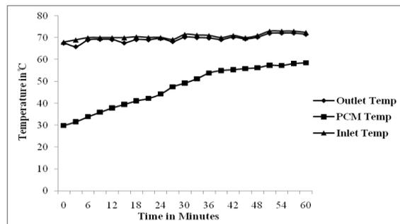
**Figure.13. Charging PCM Temperature with respect to Time for flow rate of 20 lit/hr of Palmitic acid**
