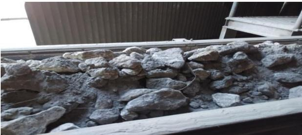
**Figure.2. Gypsum size on weigh feeder**
