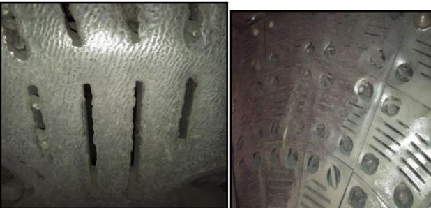
**Figure.3. Mill inner conditions**
