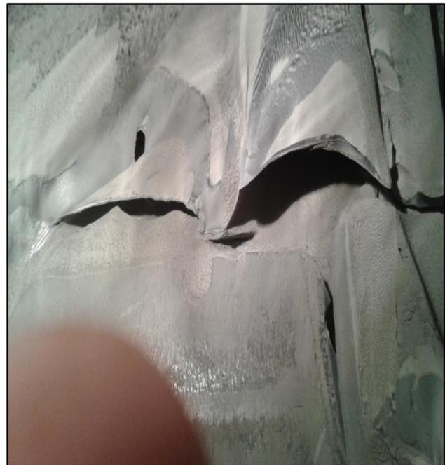
**Figure.4. Wear found in separator fan**
