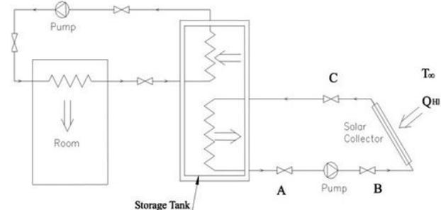
Figure.2. Schematic Diagram of the Solar Energy Storage System
