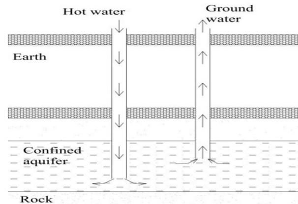
Figure.1. Underground sensible energy storage system
