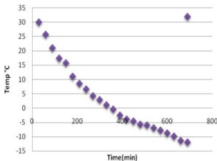
Graph .1. Freezing curve (80%water + salt 20%)
