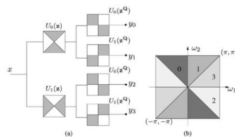
Figure.4.(a)Filtering structure.(b)Frequency decomposition
