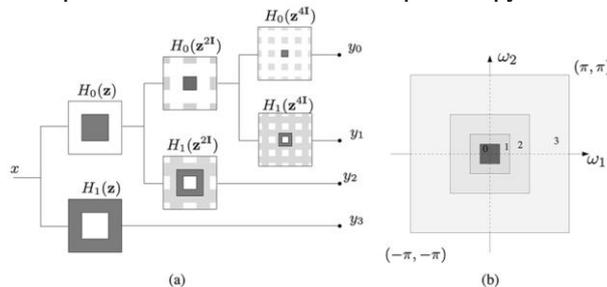
Figure.3.(a) 3 stage pyramid decomposition . (b) Subbands on the 2-D frequency plane
