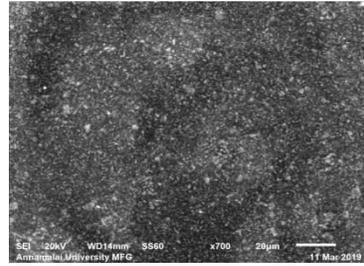
Figure.11. SEM In 700µm Before Salt Spray Test
