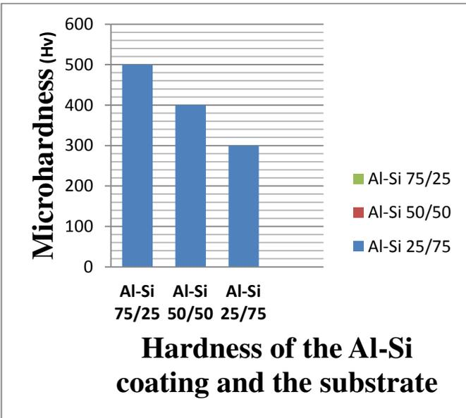
Figure.No.9. Micro hardness of the Coating
