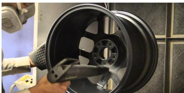
**Figure 7.2 powder coating in Automobile industry**
