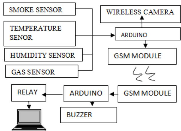
**Figure.7. Block Diagram of fire Surveillance System**
