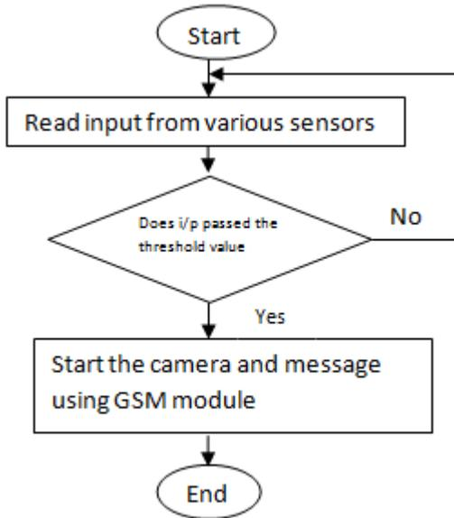
**Figure.8. Flowchart of the Transmitter Section**
