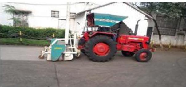
This is a new road sweeper it will be running for each and every one hour continuously.
