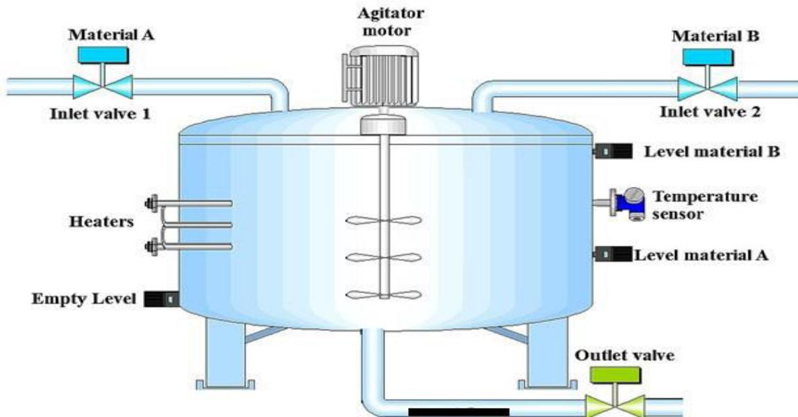
Figure.1. Automatic and Mixing of Products design diagram
