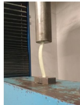
Figure .7. Plate deformed due to buckling [7]
