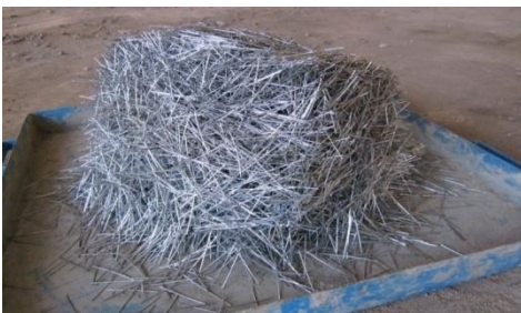
Figure.4. Galvanized iron (GI) fibers
