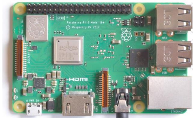
Figure.1. Raspberry Pi 3 Model B+ Hardware
