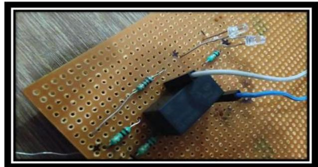
Figure .6. Overcharge Controller with Auto Cut System:-
