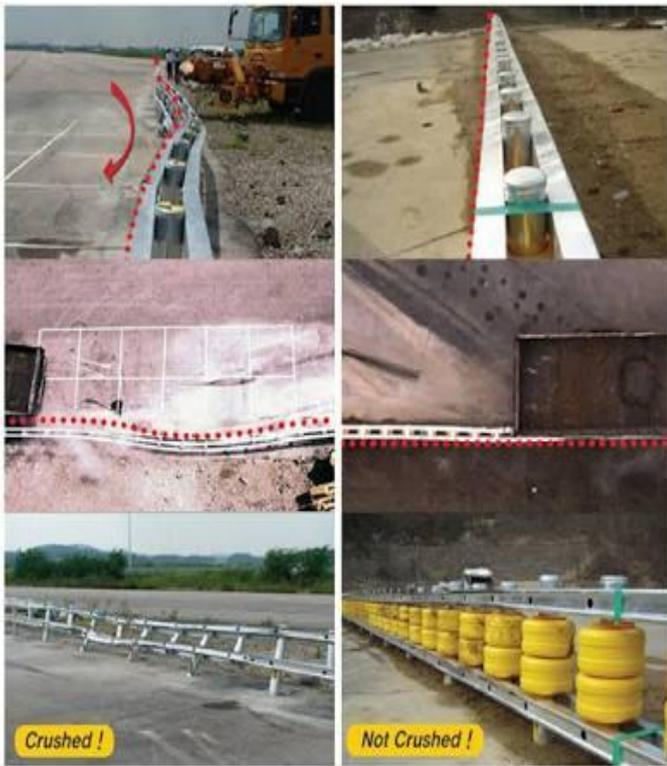
Figure.3. Working process of rolling barrier
