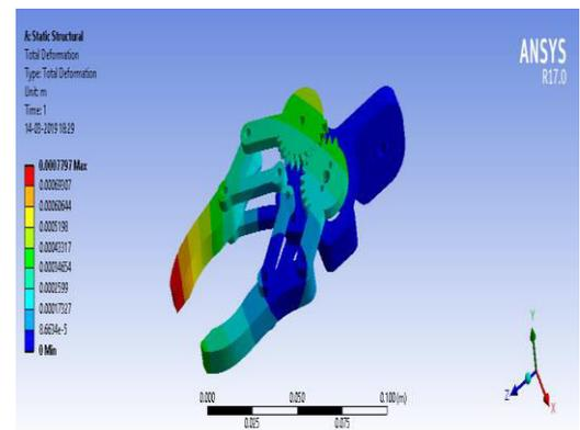
**Figure.1. Total Deformation**
