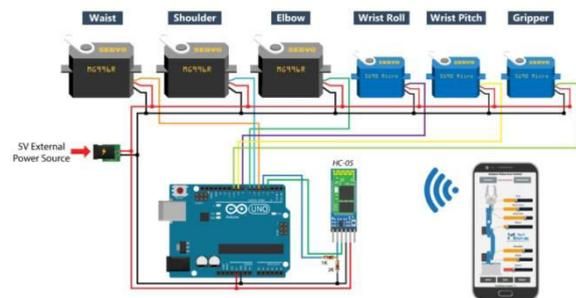
Figure.1.Design components of pick and place robot.
