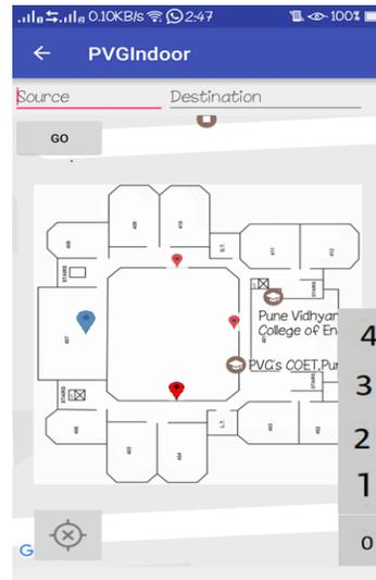
**Figure.5. Blueprint of the considered floor. Red spots refer to the access points and blue spot represents the floor located using trilateration algorithm.**
