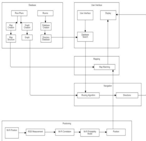
Figure. 2. Proposed Indoor Positioning System Modules
