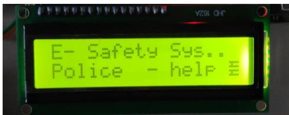
Figure.6.1 (a) LCD indication when switch 1 is activated
