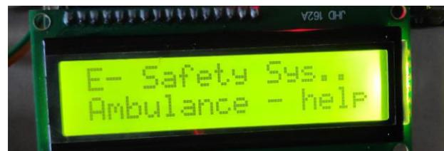
Figure.6.3. (a) LCD indication when switch 3 is activated
