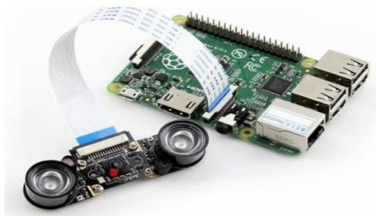
**Fig 3: Camera with night vision support.**
