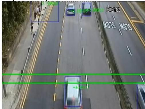
**Fig 5: An image illustrating the two reference lines for calculation of speed.**
