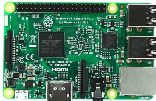
**Fig 4: Raspberry Pi: A Single board computer used for the current project**
