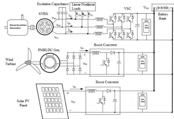
**Figure.1. Proposed single VSC and brushless generation based standalone microgrid system with GSM CONTROL STRATEGY FOR PROPOSED STANDALONE MICROGRID SYSTEM**
