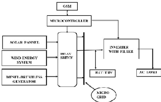
Figure.3. Block Diagram for Hybrid Diesel-Wind –PV System by using GSM Based Switch
