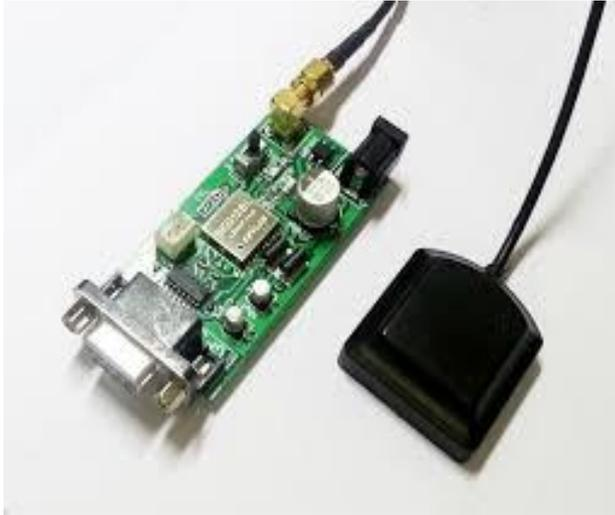
**Figure.2. GPS Receiver and Antenna**
