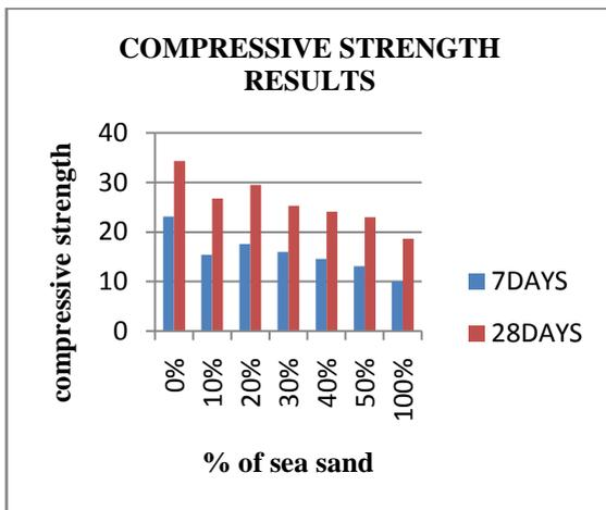
**Figure.5.2. Variation in compressive strength at 7 days & 28th day of M30 with various % of sea sand respectively.**
