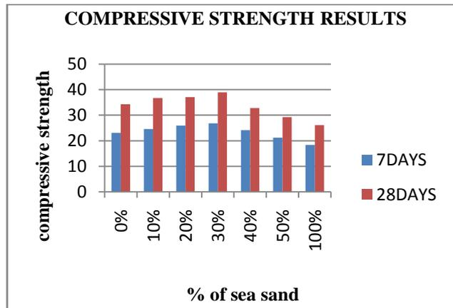
**Figure.6.2. Variation in compressive strength at 7 days & 28th day of M30 with various % of sea sand respectively (Acid wash).**
