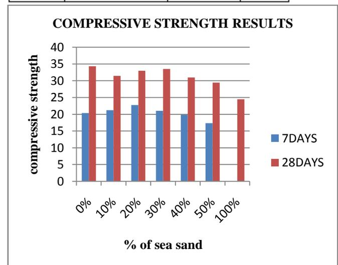
**Figure.6.1. Variation in compressive strength at 7 days & 28th day of M25 with various % of sea sand respectively (Acid wash).**
