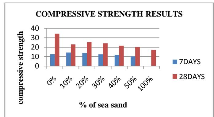
**Figure.5.1. Variation in compressive strength at 7 days & 28th day of M25 with various % of sea sand respectively.**
