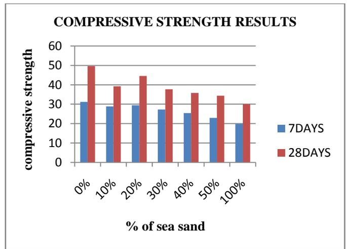
**Figure.6.3. Variation in compressive strength at 7 days & 28th day of M35 with various % of sea sand respectively (Acid wash).**
