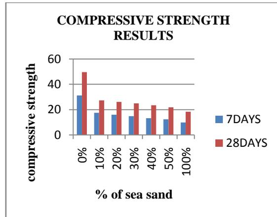
**Figure.5.3. Variation in compressive strength at 7 days & 28th day of M30 with various % of sea sand respectively.**
