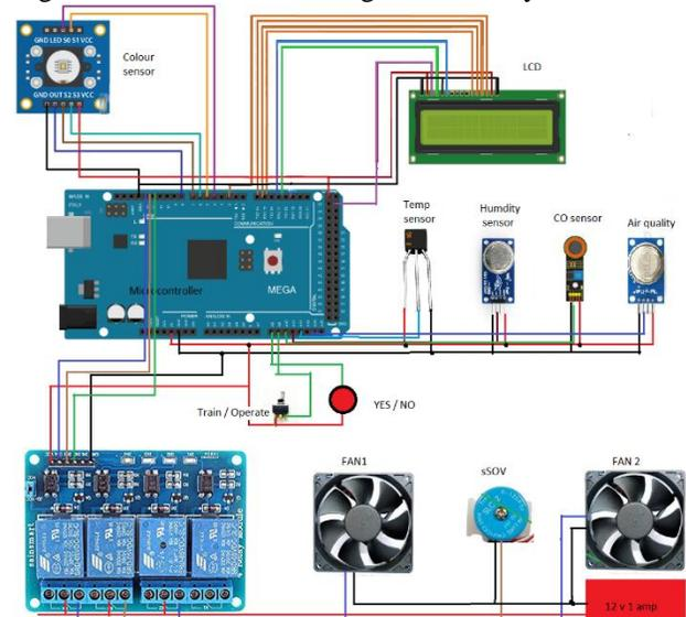
Figure.2. Circuit diagram for the e nose
