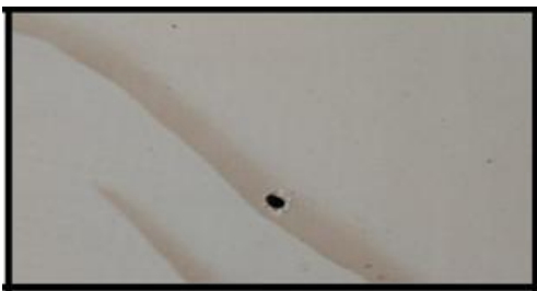
Figure.6. Drilling without tiles breakage
