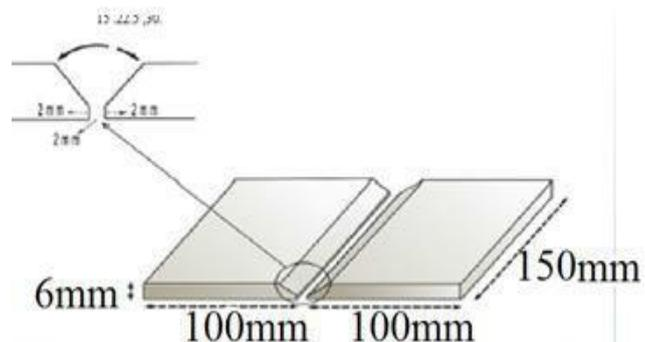
**Figure.2. dimensions of the plates for welding**
