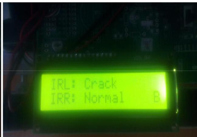
Fig 6: Left crack is detected
