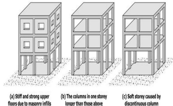
**Figure.1. Typical example of first soft storey**
