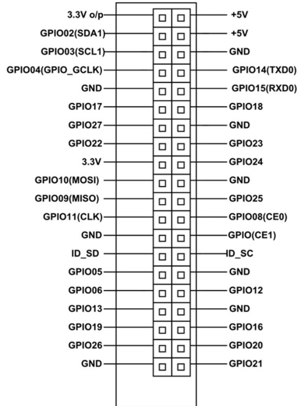
**Figure.3. Pin diagram of Raspberry Pi**
