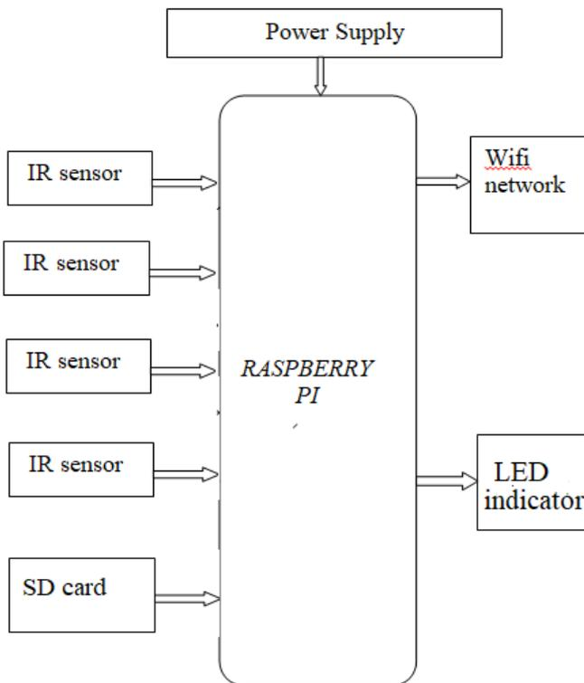
**Figure.2. Block diagram of hardware system**
