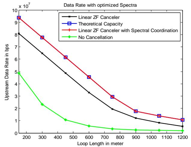
Figure 5. Data Rate with Optimized Spectra
