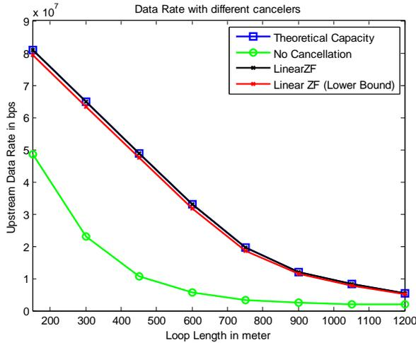
Figure 3. Data Rate with Linear ZF Canceler for Fixed Spectra
