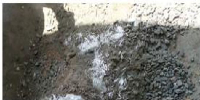
Figure.4. addition of glass fibre into mix
