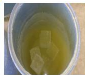
Figure.3.3 Sea Water curing
