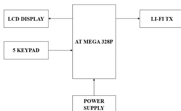
Figure .1. Block Diagram of Li-Fi Module
