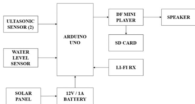
**Figure .2. Block Diagram of Shoe Module**
